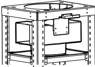
3. Measure length of 8" (20.3 cm) vent needed to connect the transition to the deflector.
