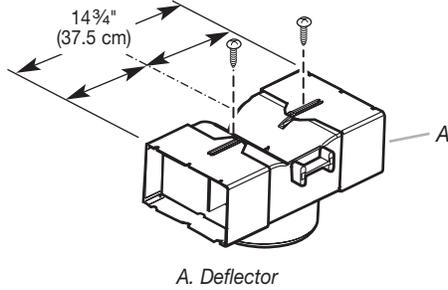
2. Attach the deflector to the bracket with 4 screws.
